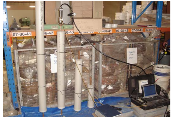
Figure 2. Bolt-grout samples tested in the laboratory
