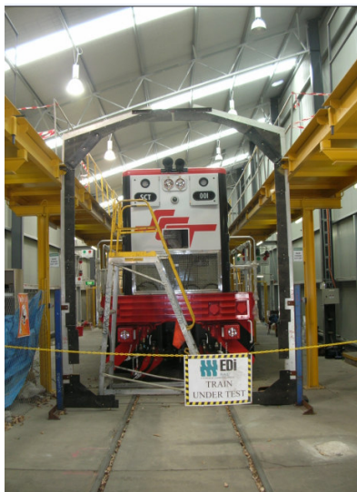
Figure 5: Locomotive being tested for gauge
