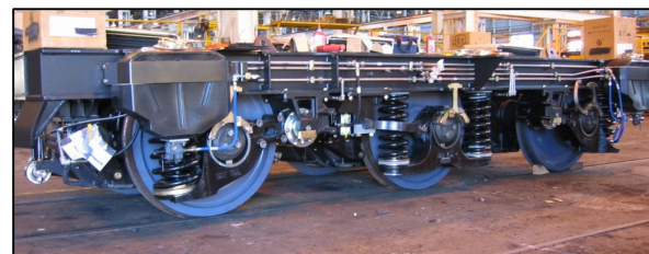
Figure 10: Semi Steering Bogies as fitted to the SCT locomotive
